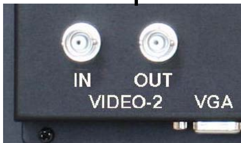
(option) BNC Video IN & loop out
